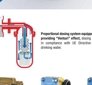
Proportional dosing system equipped with device providing "Venturi" effect, dosing polyphosphate in compliance with UE Directive 98/83/CE for
