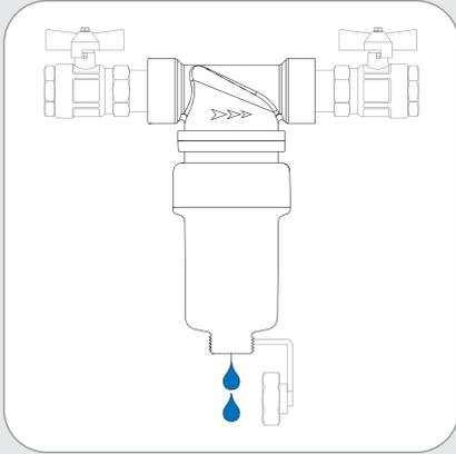
FDM-2 must be always installed in the upright position. It is recommended the installation of shut-off valves before and after FDM-2.
