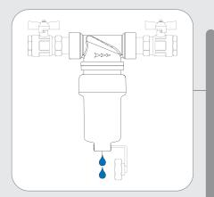
FDM-2 must be always installed in the upright position. It is recommended the installation of shut-off valves before and after FDM-2.
